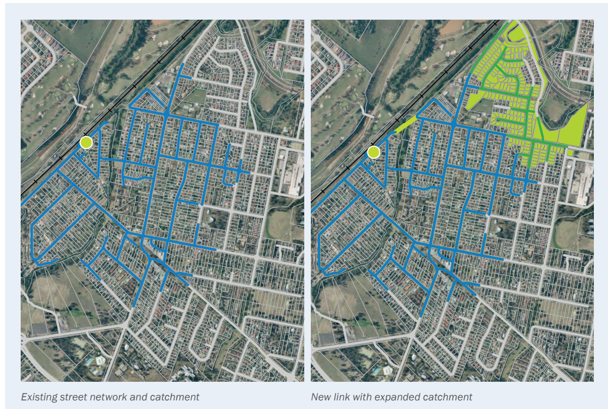
Figure 3.2 Expanding a public transport catchment by completing a missing link
